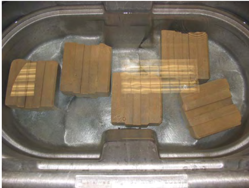
Photo No. 1 Standard Brick Water Absorption Setup
