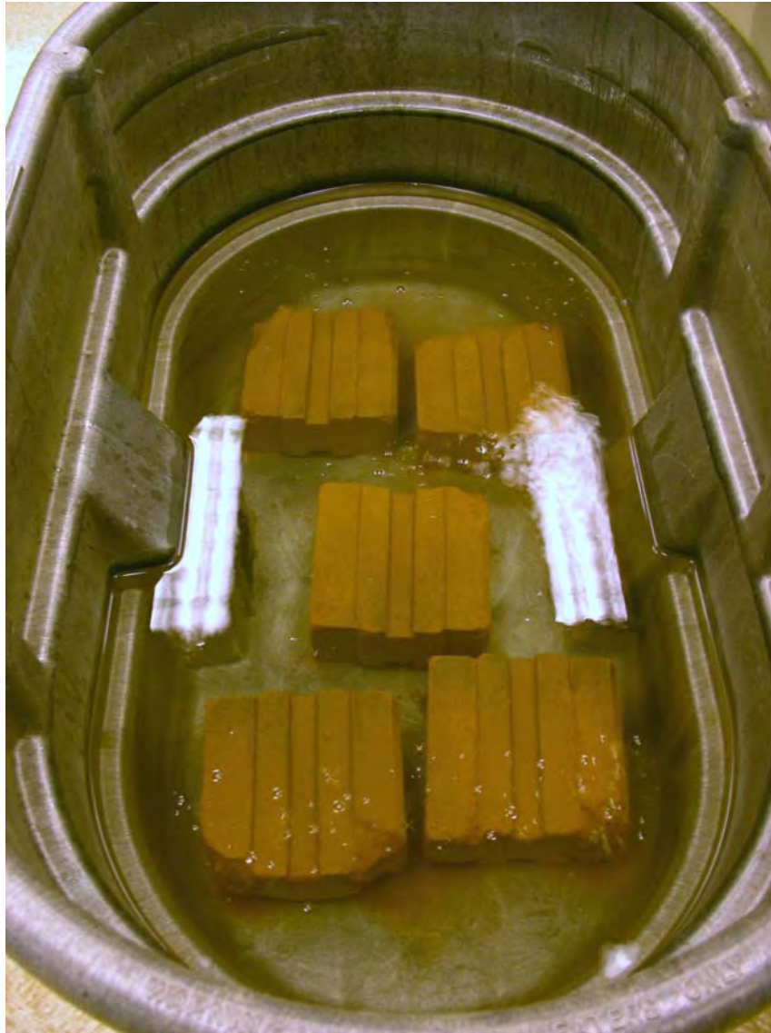
Photo No. 2 F-Series Brick Water Absorption Setup
